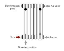
The flow must be connected on the side closest to the flow diverter
